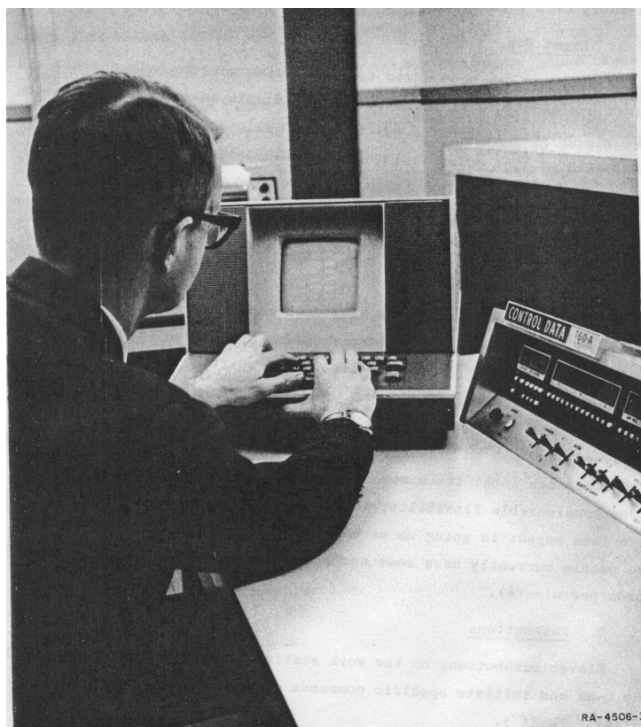
Figure 1. Control Data CDC-160A workstation at SRI. For this interactive workstation, operators used Engelbart's five-key "chordal" keyset (not shown) that allowed one hand to type while the other used a light pen. (Courtesy of SRI International)
