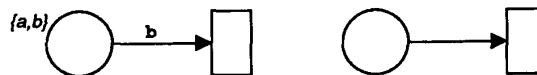
Figure 1: A very small coloured Petri net, and its skeleton (without initial markings)
