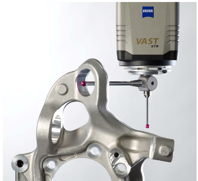
Fig. 3. Complex geometry is difficult to measure by CMM without multiple time-consuming repositioning and reconfiguration (source: www.zeiss.de)
