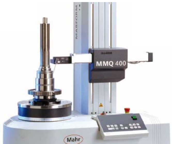
Fig. 1. Marform roundness tester has rotating table with limited capabilities of measured object manipulation (source: www.mahr.de)
