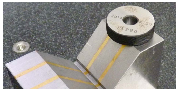
Fig. 6. The measurement gauge (internal diameter D = 10.998 \text{ mm} ) used as measured object, attached in fixed position by magnetic holder.
