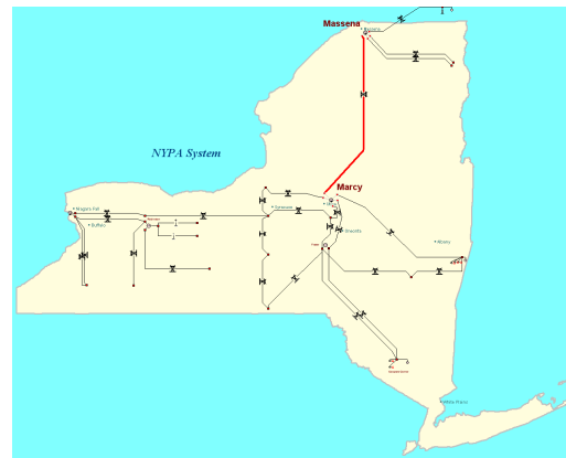
Figure 7. One-Line Diagram of NYPA Test System Superimposed on NY State Map.
