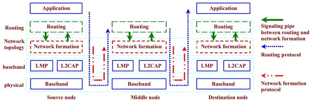
Fig. 3 A simplified Bluetooth GN protocol stack
