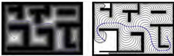
Fig. 3. Left - Slowness map and the path obtained with FM2 Right - Wavefronts at each iteration. The path is perpendicular to each front wave.
