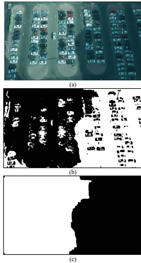
Fig. 5. Shade Detection. (a) Image with non-uniform lighting. (b) Detect region with shade. (c) Final separation of the two region.
