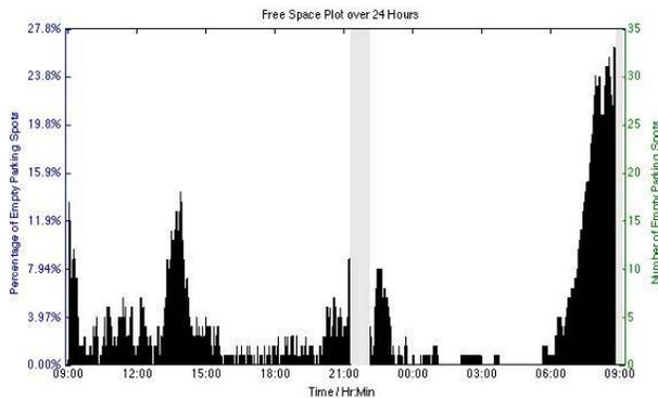
Fig. 8. Free space plot over 24 hours. The number of free parking spots over time, out of 126 total spots.
