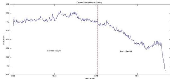
Fig. 6. Contrast value over time. Contrast value declines rapidly in insufficient sunlight.
