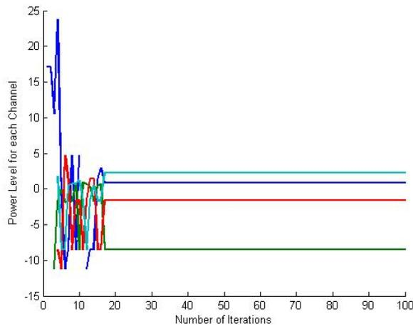
Figure 4: Plot of the Transmit Power for Power Control game
