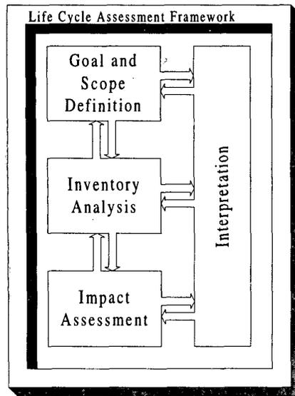
Figure 2. The LCA Framework according to ISO 14040 (adapted from [4])
