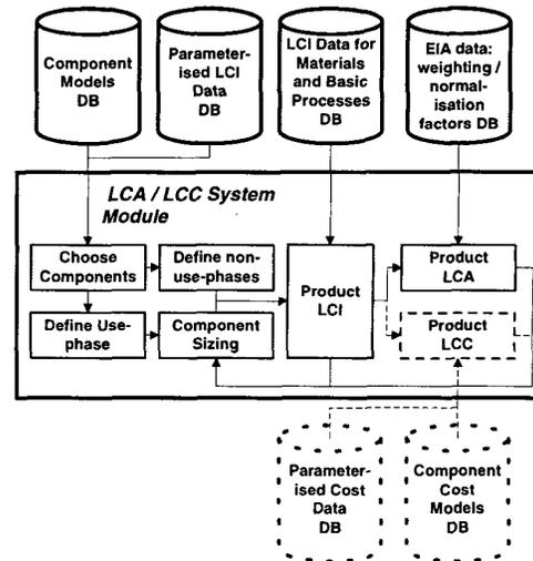
**Figure 4. General Flowchart of LCA/LCC System Module and required databases**
