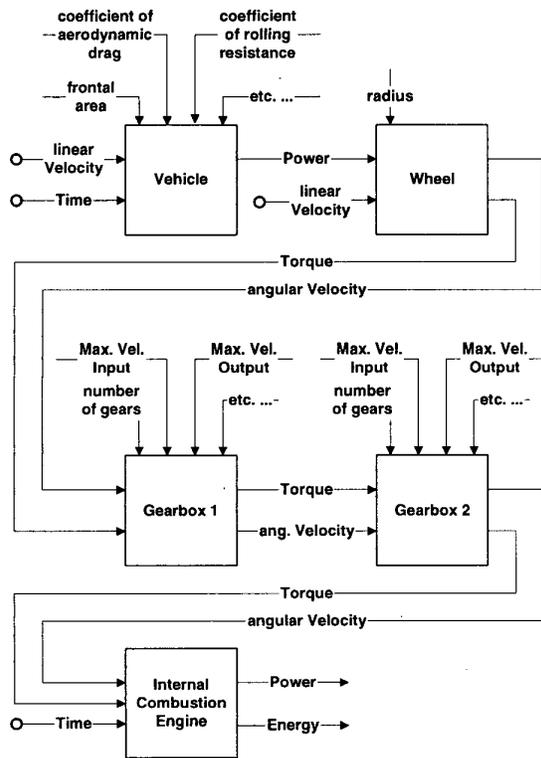
**Figure 6. Example: Flowchart of a Vehicle illustrating linked Components for the use-phase**
