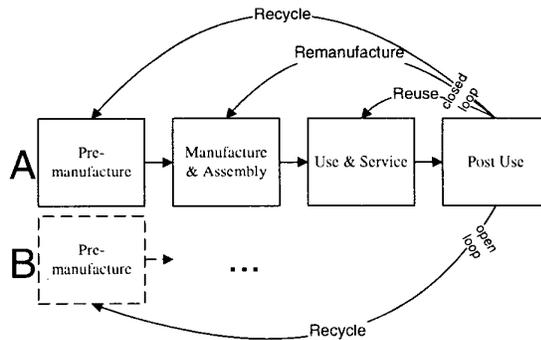
Figure 1. Simplified schematic of Life Cycle Stages illustrating recycling (open- and closed-loop), remanufacturing and reuse.
