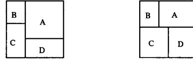
Figure 2: These two floorplans represent two distinct rectangular topologies. Note the variations in the block surrounds.
