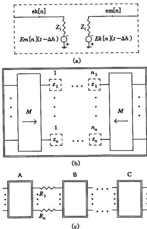
Fig. 4. (a) Equivalent impedance network of a section of one of the lossless decoupled lines. (b) Equivalent network of  $n$  lossless coupled lines using the model of (a). (c) Equivalent network of  $n$  lossy coupled lines using the model of (b).
