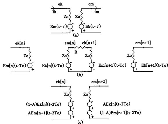
Fig. 1. (a) Equivalent impedance network of a lossless transmission line (b) Equivalent impedance network of a lossy transmission line (c) compacted version of (b).
