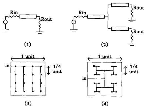
Fig. 2. Four lossy transmission line configurations. Configurations (3) and (4) connect sixteen equally spaced points on a one unit by one unit surface. For configurations (3) and (4),  $s$  is the number of sections in a  $1/4$  unit length conductor and  $R_t$  is the total series resistance of a 1 unit length conductor.
