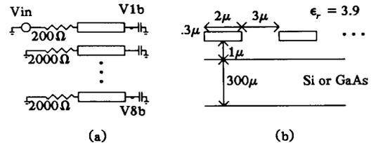
Fig. 7. (a) Eight parallel transmission lines of coupled length .5cm terminated in  $20fF$ . (b) Cross sectional view of the conductors.
