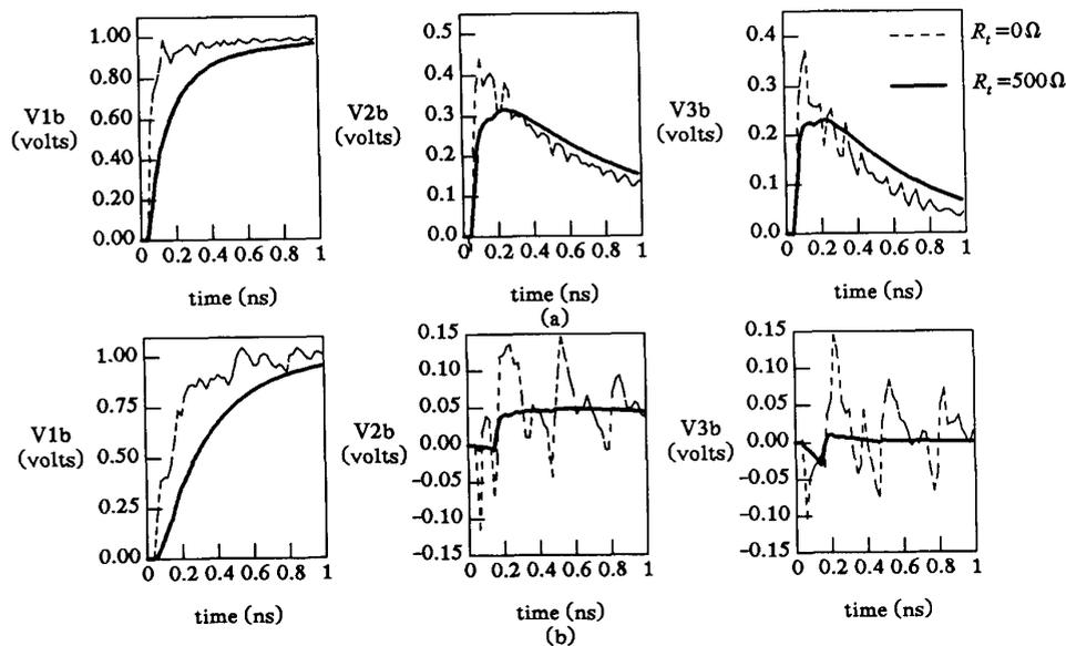
Fig. 8. Voltages at the endings of three of the eight lines shown in Fig. 7 with and without the series resistance included. (a) gallium arsenide (b) silicon. The input rise time is 10 psec.
