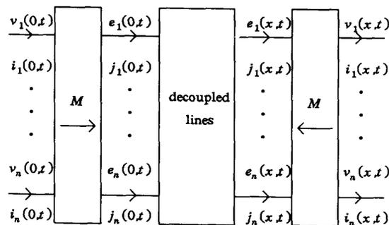
Fig. 3. Equivalent representation of  $n$  coupled lines of coupled length  $x$ . The boxes labeled  $M$  represent transformation networks.
