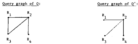
Figure 2.1: Two equivalent queries, one having a cyclic query graph and the other a tree query graph.
