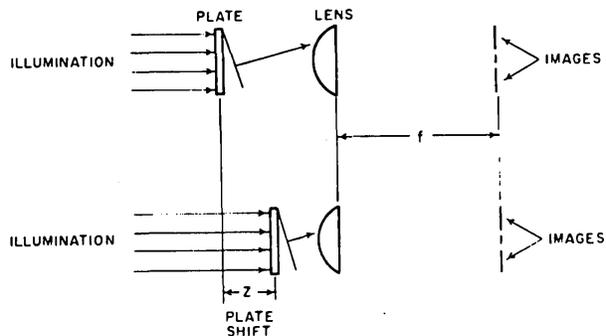
Figure 7—Z axis displacement, Fraunhofer hologram
