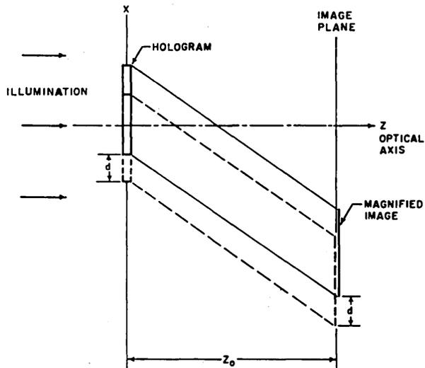
Figure 4—Lateral shift of plate, Fresnel hologram
