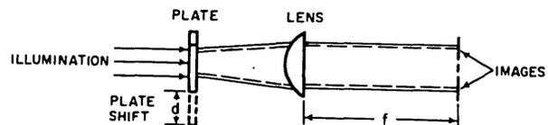
Figure 8—X or Y axis displacement, Fraunhofer hologram
