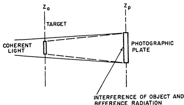
Figure 1—Holographic construction
