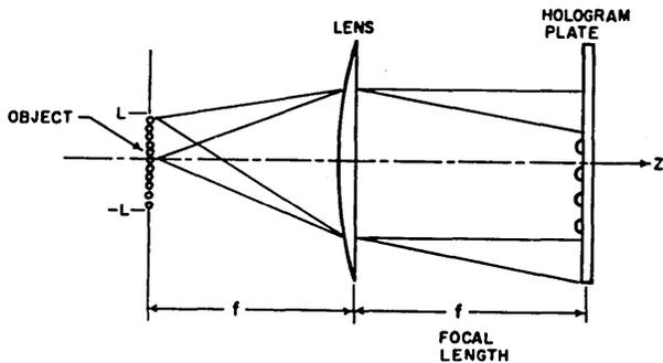
Figure 5—Construction of object at infinity
