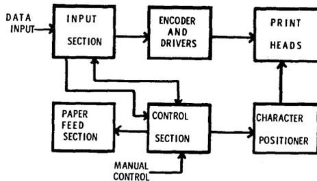
Figure 6—Printer block diagram
