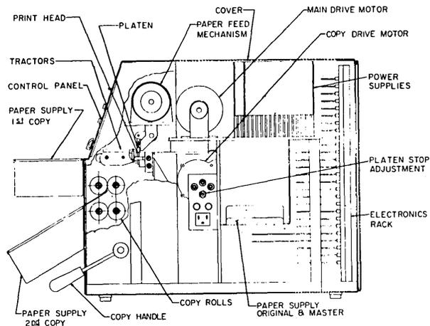
Figure 7—Printer layout
