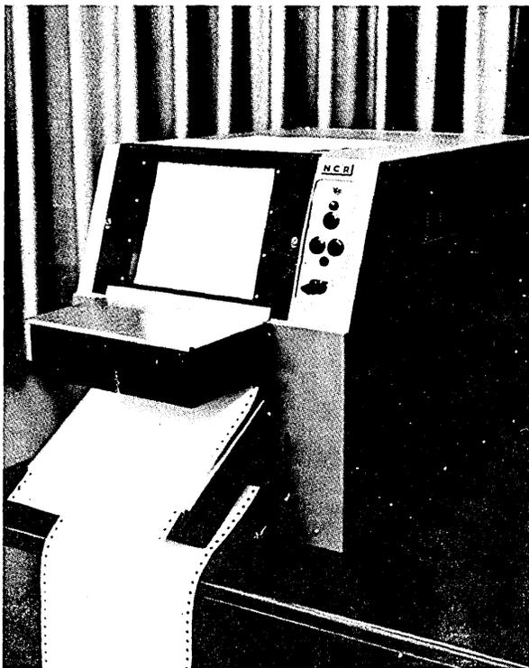
Figure 8—High-speed thermal teleprinter
