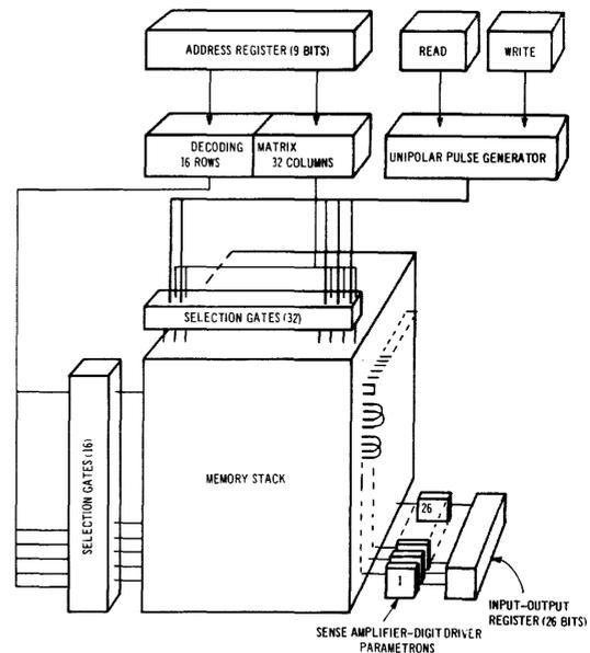
Figure 10. Block Diagram of 512 Word, 26 Bit/Word System.
