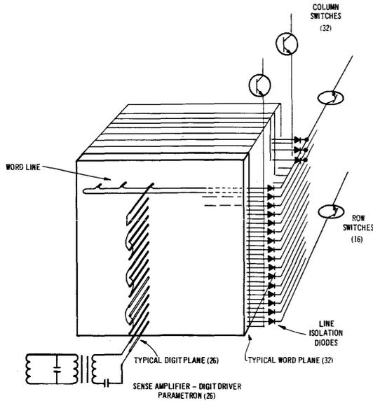
Figure 6. Stack Arrangement.
