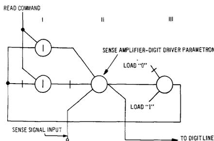
Figure 12b. Sense Amplifier-Digit Driver and Input-Output Register Logical Diagram.
