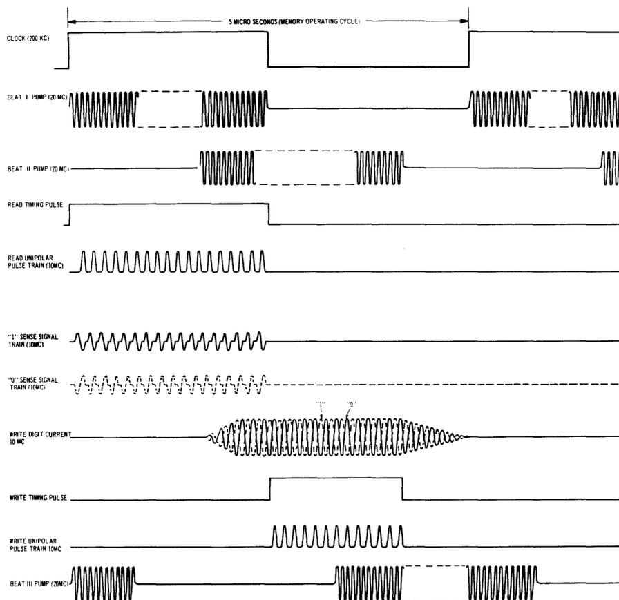
Figure 13. Memory Cycle Timing.
