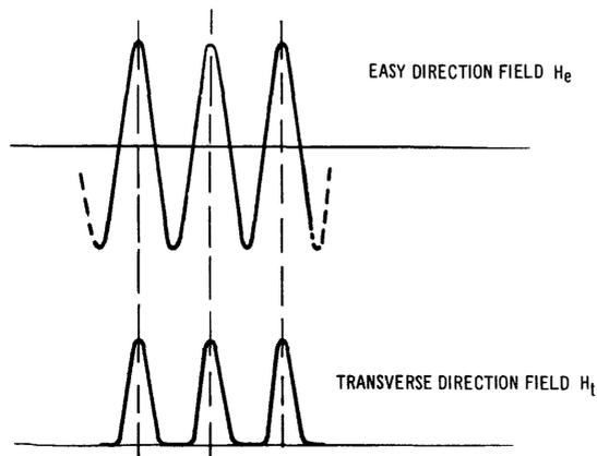
Figure 1. Unipolar  $H_t$  Pulse and Sinusoidal  $H_e$ .
