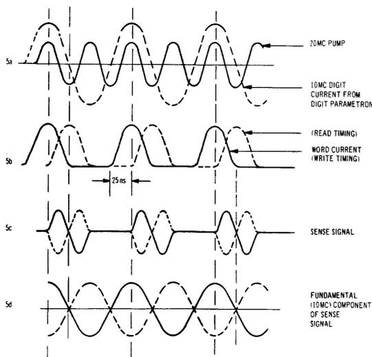
Figure 5. Timing Relations for Read-Out Phase Correction.
