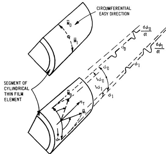
Figure 3. Derivation of Readout Signal.
