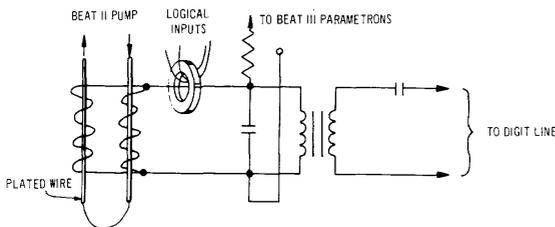
Figure 12a. Sense Amplifier-Digit Driver Parametron Schematic.
