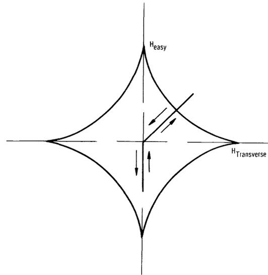
Figure 2. Locus of Applied Field During Write Cycle with Unipolar  $H_t$ .
