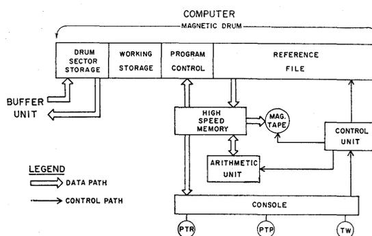
Fig. 6—Block diagram of the Recorder Central.
