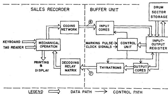
Fig. 5—Block diagram of the Buffer Unit.
