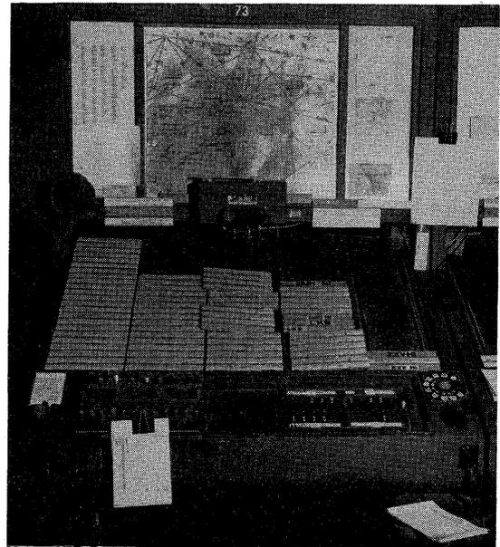
Fig. 2—Flight-progress board.
