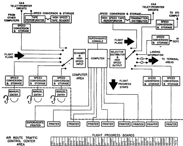
Fig. 6—Block diagram of prototype data-processing system.
