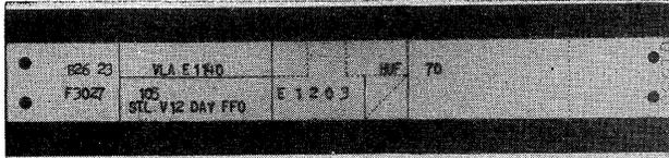
Fig. 4—Automatically prepared flight-progress strip.
