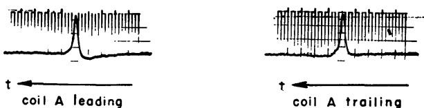
Fig. 7. Actual wave forms showing effect of direction of surface motion
