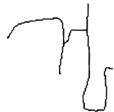
6(e) Result of linking the same road with curvature checking. Parameters: w_{smooth}=9 , w_{non-smooth}=10 , w_{angle}=100 , w_{grey-scale}=0 , w_{curvature}=40 .
