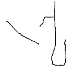
6(d) Result of linking one road without curvature penalty. Parameters: w_{smooth}=9 , w_{non-smooth}=10 , w_{angle}=100 , w_{grey-scale}=40 , w_{curvature}=0 .
