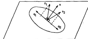
Figure 11: A diagram showing how two similar and shifted rows of the image are mapped to vectors with opposite directions.
