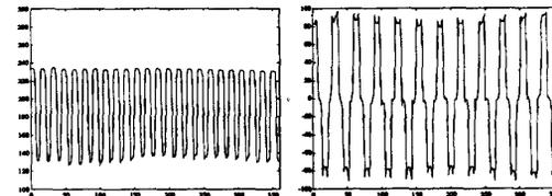
Figure 12: (a) Result of simple projection of the image of Fig. 9 along horizontal axis. (b) Result of applying the projection after preprocessing the image (see text).
