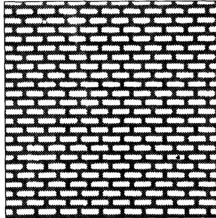
Figure 9: An image from a chip with similar and shifted rows.
