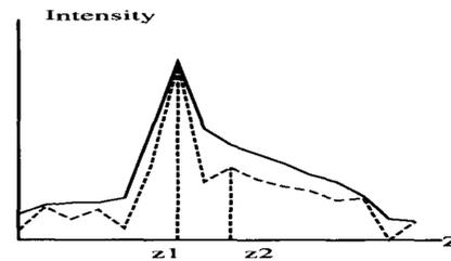
Figure 6: This figure shows the signal resulting from two surfaces at heights  $z_1$  and  $z_2$ . The curve in solid lines represents the original signal. Note that the surfaces at  $z_1$  and  $z_2$  are close enough for their responses to overlap. This causes the original signal to contain only one peak. The result after applying deconvolution (Wiener filtering) is shown in dashed lines. Note that we have now resolved the two peaks at  $z_1$  and  $z_2$ .
