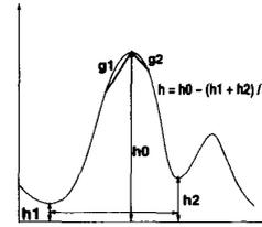
Figure 5: Peaks and valleys are identified through changes in the sign of the gradient. The height of a peak is defined to be the average height above the two neighboring valleys (minima).
