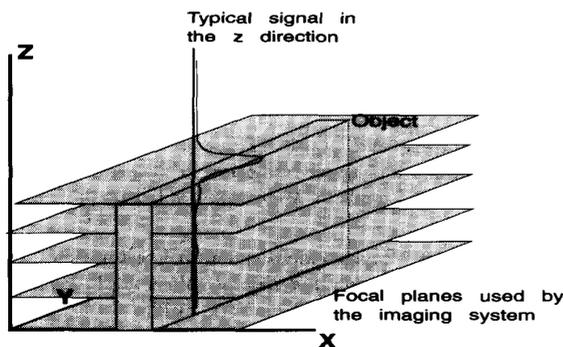
Figure 4: Numerous confocal image slices are stacked along the z-direction, which is parallel to the optical axis. The object being imaged is a thick metal line, whose top surface causes a peak in the intensity signal measured along the z axis.
