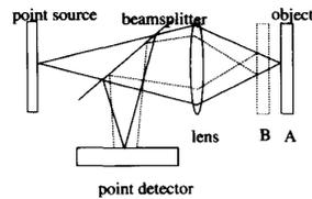
Figure 2: Imaging of the object using a confocal microscope. At position A the object is in focus, while at B it is defocused.
