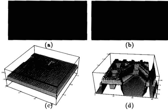
Figure 11: The result of applying Wiener filtering followed by peak detection and smoothing. Height is encoded via intensity. (a) The upper height image; (b) The lower height image. (c) and (d): A wireframe plot of the surfaces.
