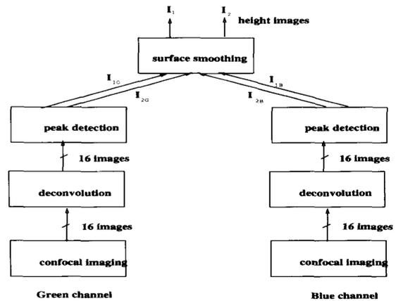
Figure 7: The block diagram of the system with the various processing stages shown. The objective of the process is to obtain two height images that can be used for further evaluation
