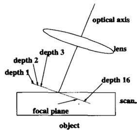
Figure 3: Illustrating the principle of tilted scanning
