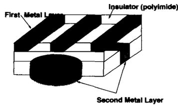
Figure 1: A schematic of the part to be inspected
