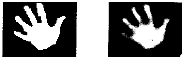
Figure 3: An example (containing preprocessing errors) of a binary image of the hand and the image reconstructed using the extracted Zernike moments through order = 25 .
