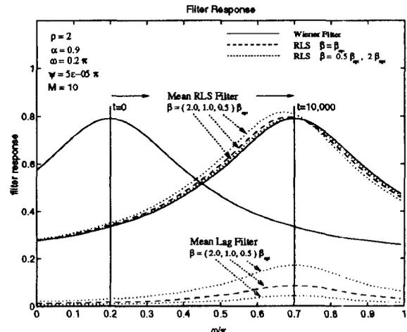
Figure 1: Filter transfer function over time for a chirped AR1 process.
