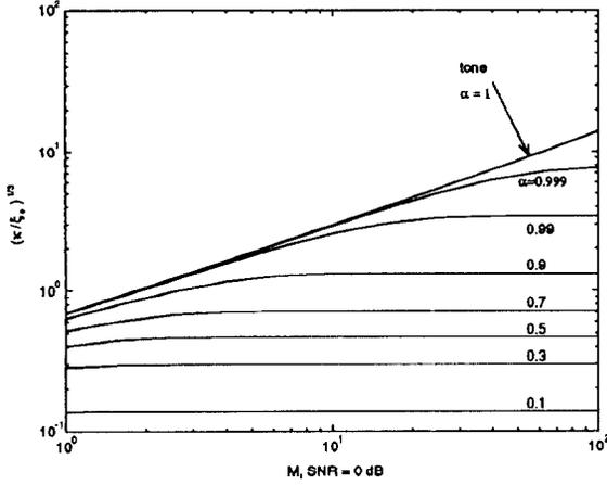
Figure 3: The signal dependent parameter  $(\kappa/\xi_0)^{1/3}$  of  $\beta_{opt}$  versus the filter length ( $M$ ) at SNR = 0dB for an AR1 process.
