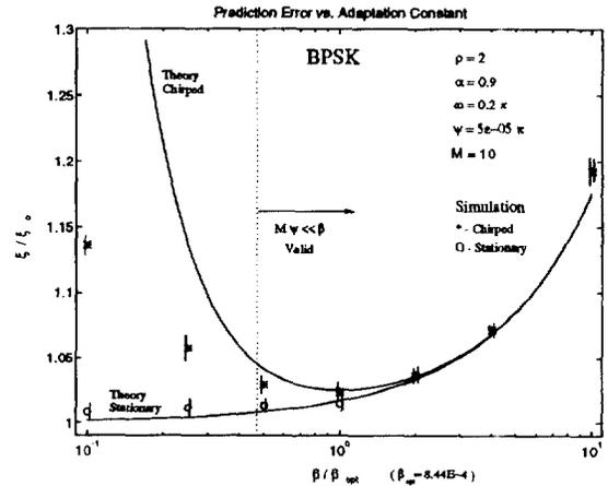
Figure 6: Misadjustment ratio ( $\xi/\xi_0$ ) vs. adaptation constant  $\beta$  for a chirped BPSK signal.
