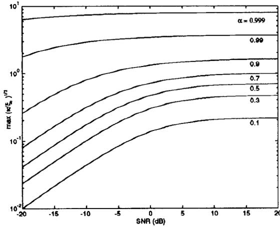
Figure 4:  $\text{Max}_M (\kappa/\xi_0)^{1/3}$  vs. SNR for an AR1 process.
