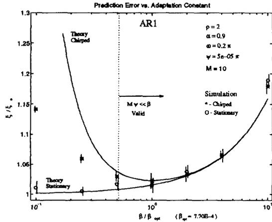
Figure 5: Misadjustment ratio ( $\xi/\xi_0$ ) vs. adaptation constant ( $\beta$ ) for a chirped AR1 process.
