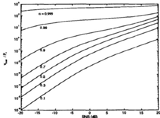
Figure 2: Normalized lag misadjustment  $\kappa_{max}/P_n$  vs. SNR for various AR1 correlation values ( $\alpha$ ) and  $M \rightarrow \infty$ .
