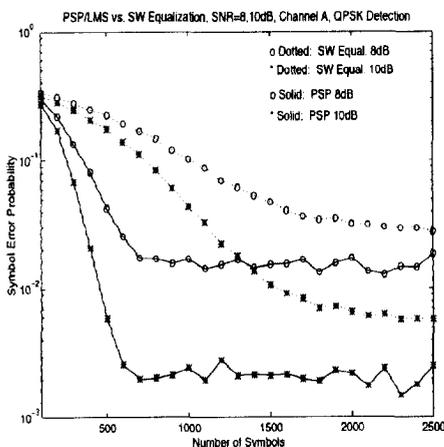
Figure 3: Unknown Channel A, PSP/MLSE vs. SW Blind Equalizer, QPSK Detection Performance
