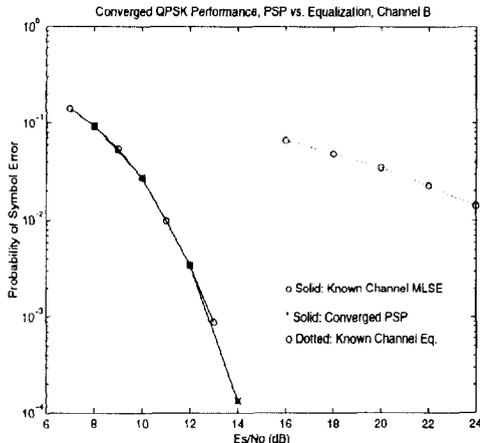
Figure 5: Converged & Known Channel QPSK Detection Performance, Channel B, PSP only
