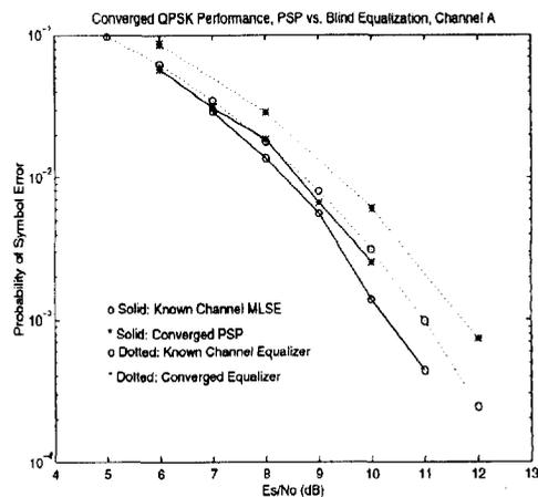
Figure 4: Converged & Known Channel QPSK Detection Performance, Channel A, PSP vs. SW
