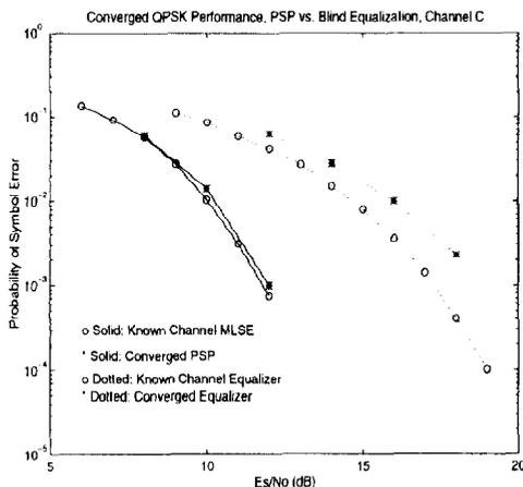
Figure 6: Converged & Known Channel QPSK Detection Performance, Channel C, PSP vs. OCMA
