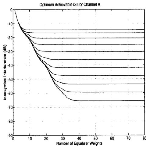
Figure 1: Equalizer Length vs. ISI, Channel A
