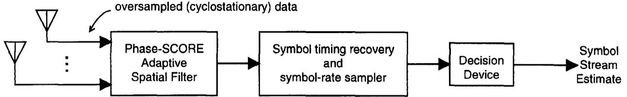
Figure 1: Block diagram of one-step blind adaptive spatial filter system.
