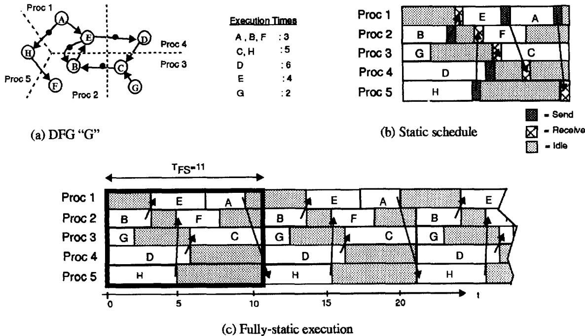
Figure 1. Fully-static schedule on five processors
