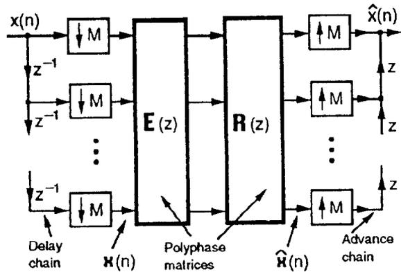
Fig. 1.1. The polyphase representation of a filter bank.
