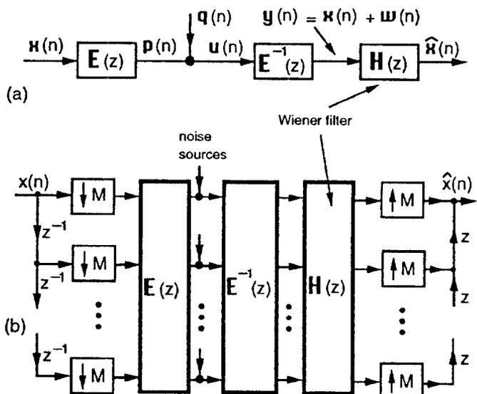
Fig. 1.3. Decomposing the synthesis bank into two parts. (a) Block diagram, and (b) internal details.
