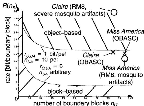
**Fig. 5.3 Data rate in bit/boundary block for predictive coding of MC-objects ( $M=0.5$ ) and different rates  $r_{C,UA}$  for coding color parameters in bit/pel. Crosses and circles mark the data rates which object-based and block-based coders spent for coding boundary blocks.**
