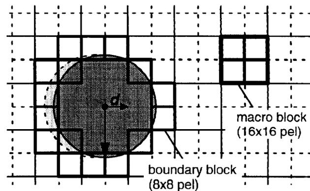
**Fig. 3.1** A circle is moving with a displacement  $d$ . The areas uncovered due to object motion are marked in a light grey. The image is divided into macro blocks consisting of four blocks. The marked blocks on the boundary of the circle are boundary blocks containing two differently moving objects.
