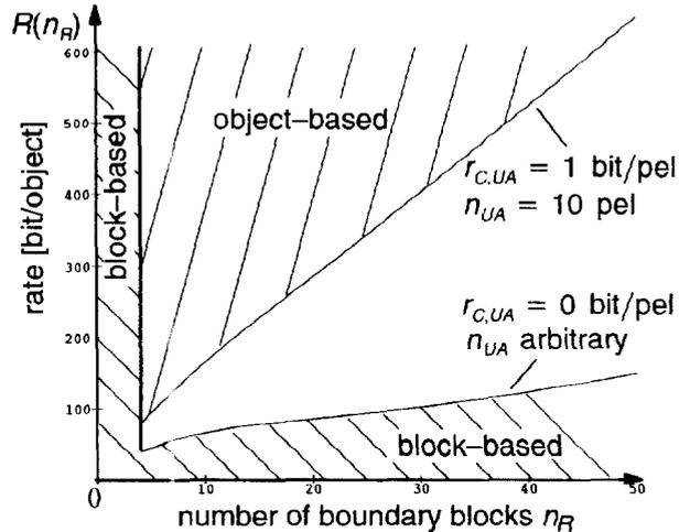
**Fig. 5.2** Data rate  $R^O(n_R)$  in bit/object. Shape parameters of MC-objects are predictively coded ( $M=0.5$ ). Color parameters of uncovered areas are coded with different rates  $r_{C,UA}$  in bit/pel.
