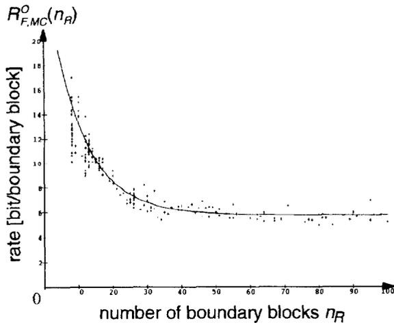
**Fig. 5.1** Data rate in bit/boundary block for coding the shape parameters of a object during its first occurrence (intra mode) as function of the object size represented by the number of boundary blocks  $n_R$ . The solid curve is the model curve according to Eq. (5.4) with  $M=1$ . In case of predictive coding the data rates have to be divided by two ( $M=0.5$ ). For the test sequences *Claire* and *Miss America*, the no. of boundary blocks is  $n_R=87$  and  $n_R=95$ , respectively.
