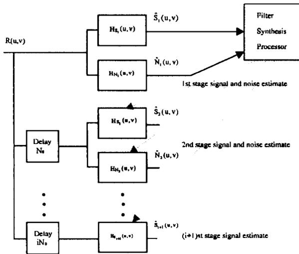
Figure 1 Block diagram of adaptive aposteriori Wiener
