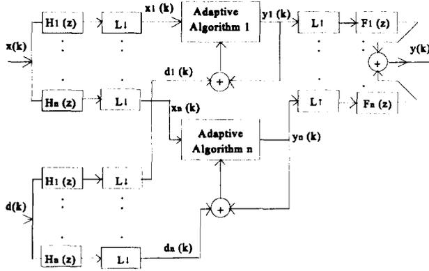
**Figure 1: Basic  $n$  Channel Adaptive Filter Bank**
