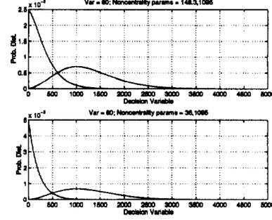
Figure 2: Probability distributions for decision metrics corresponding to assumed correct and incorrect timing estimates.  $\sigma_\eta = 80$
