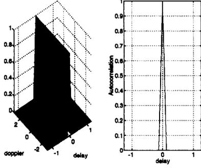
Figure 1:  $Ideal|\chi(\tau - \hat{\tau}, \nu)|^2$  for  $\nu \in [-\Omega, \Omega]$ . Delay and Doppler axes normalized
