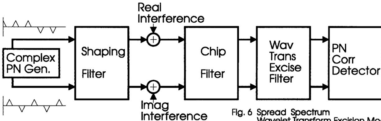
Fig. 6 Spread Spectrum Wavelet Transform Excision Model
