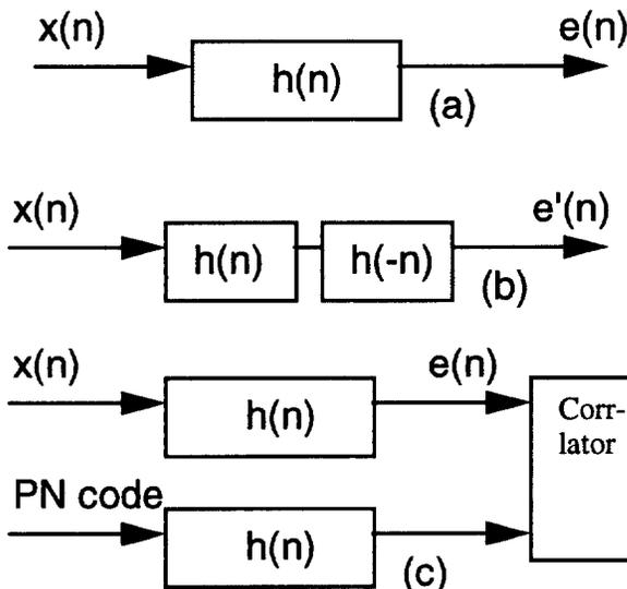
Fig.5 Match filter structures
