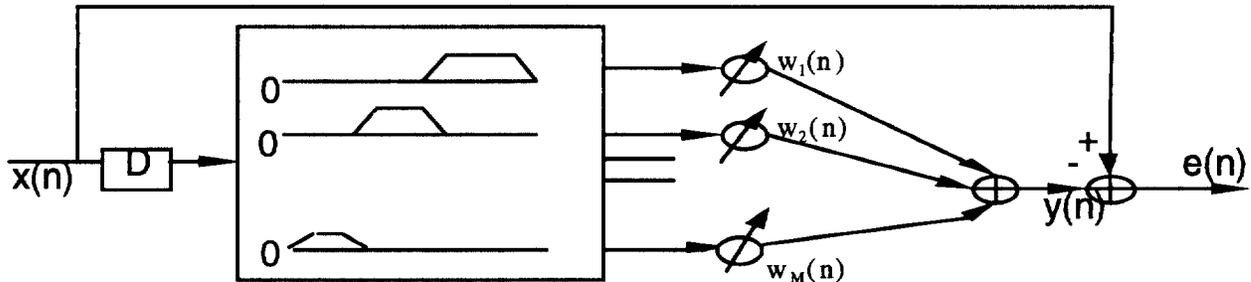
Fig.4 M-band wavelet filter banks
