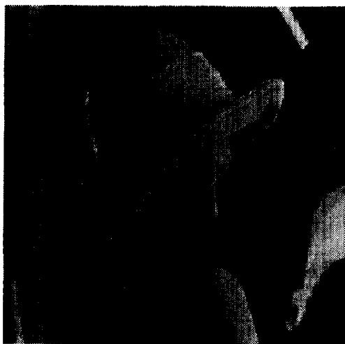
Figure 4: GTSLVQ Compressed Image at 0.5 b/pixel, 4x4 blocks, PSNR = 28.38 dB
