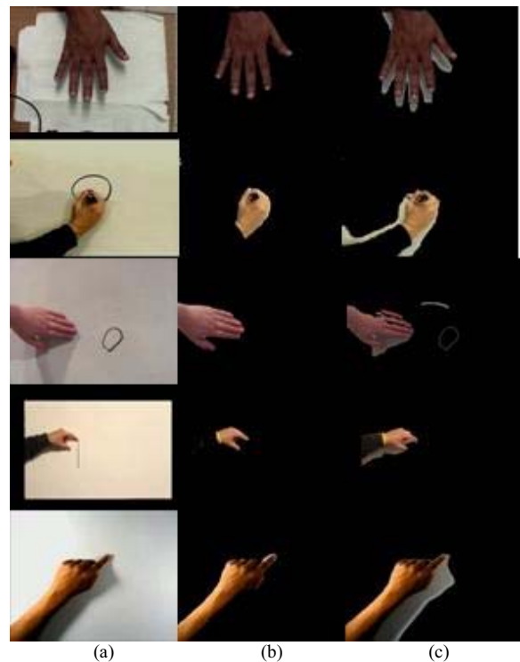
Figure 3. show the result of background subtraction based on our proposed method and OpenCV Gaussian mixture model; (a) is the original images, (b) is background subtraction using our proposed method and (c) is the background subtraction using OpenCV Gaussian mixture model.
