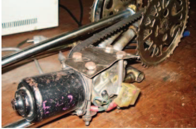
Figure 6: Motor connected to sprockets with timing belt
