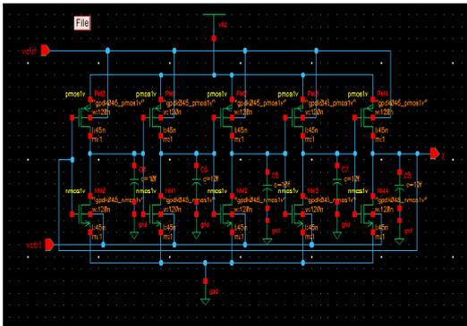
Figure 6 VCO with reverse substrate bias technique.
