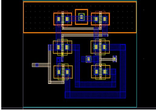
Figure 2 Layout of VCO Ring oscillator.
