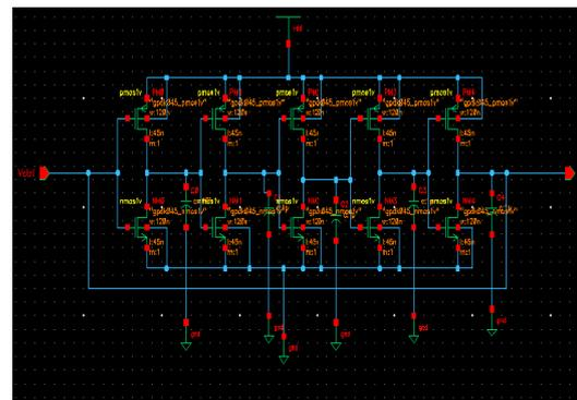
Figure 1 Five stage VCO ring oscillator
