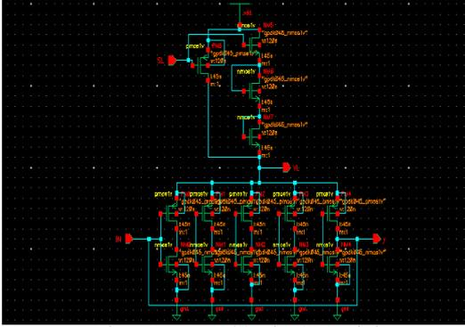
Figure 5 VCO using SAL technique.
