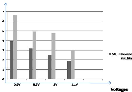
Figure 8 Oscillation frequency of VCO ring oscillator
