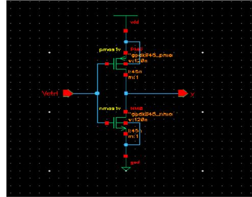
Figure 4 Gate level Inverter design
