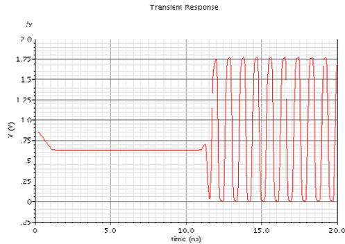
Figure 3 Waveform of VCO Ring oscillator.
