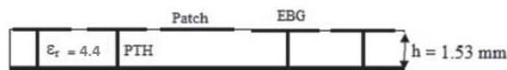
Fig. 9 Side view of EBG structure with microstrip hexagonal patch in the same plane
