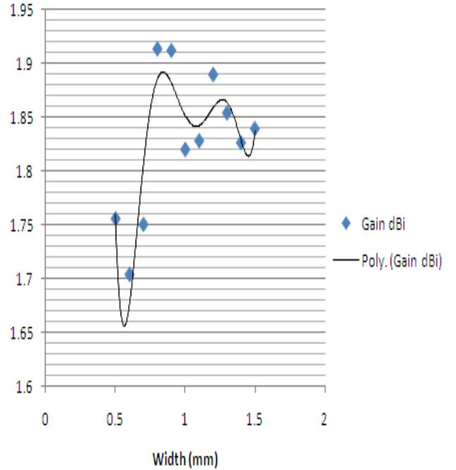
Fig.6: Plot of Gain (Y-axis) vs Width (X-axis) of the slot.
