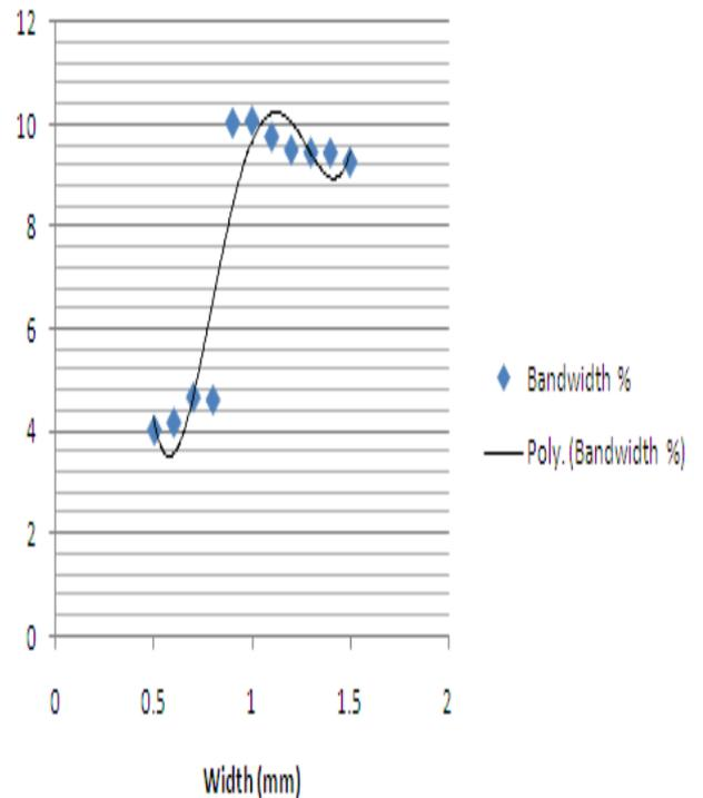
Fig.7: Plot of Bandwidth (Y-axis) vs Width (X-axis) of the slot
