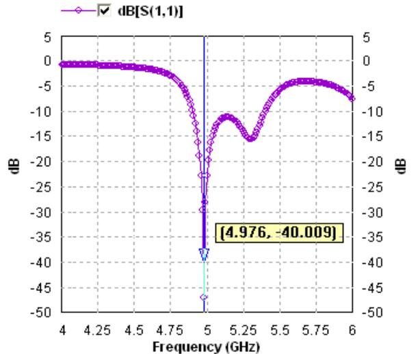
Fig.4 (b): Simulated Return Loss for Slotted Triangular MPA
