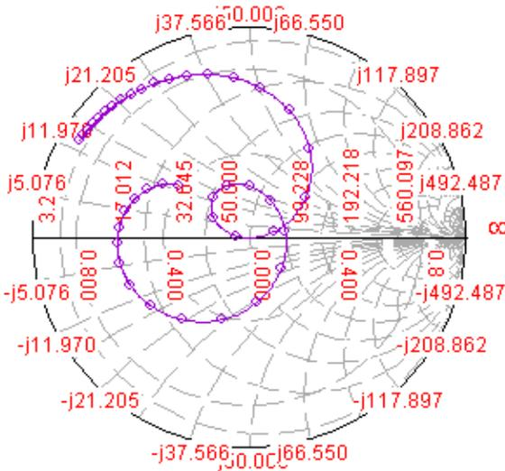
Fig.5 (b): Smith Chart for Slotted Triangular MPA.
