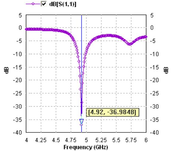
Fig.4 (a): Simulated Return Loss for Triangular MPA
