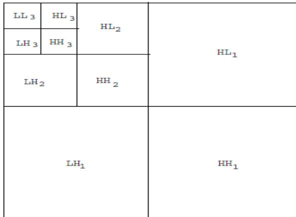
Fig2. DWT pyramid decomposition of an image
