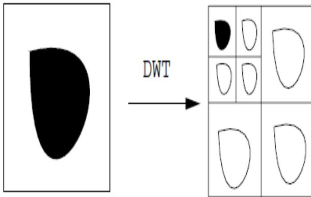
Fig3. Example of DWT pyramidal decomposition
