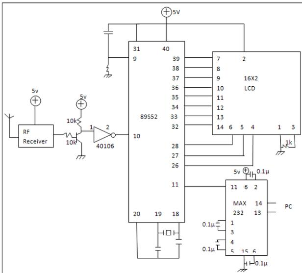
Figure C: Block diagram output circuit with receiver.
