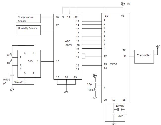
Figure A: Block diagram of wireless sensor node
