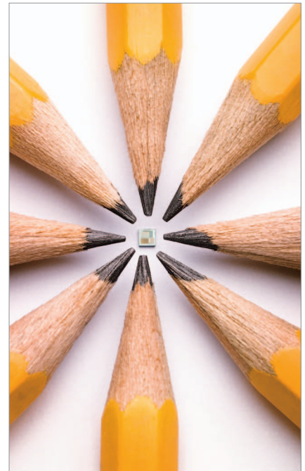
Figure 7. Hewlett-Packard Labs has developed a 2–4 mm square wireless chip that can store up to several Mbytes of data.
