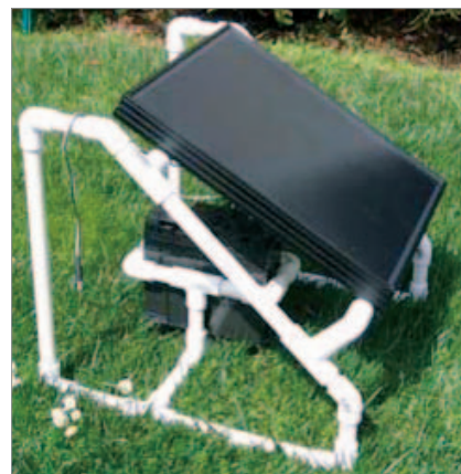
Figure 4. A Green WiFi prototype assembled using a PVC frame is undergoing testing in San Francisco.
