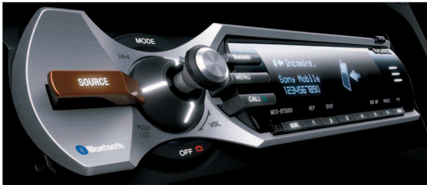
Figure 5. Sony's MEX-BT5000 audio head unit seamlessly integrates any Bluetooth-enabled mobile phone with the car's audio system, letting you make and receive calls without touching the phone.
