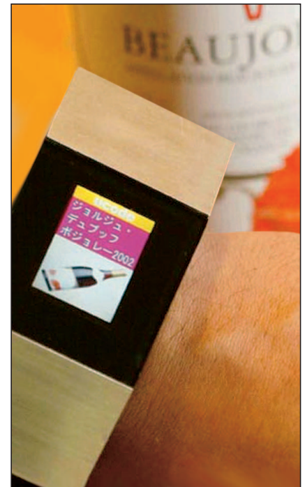
The watch-style version of the Ubiquitous Communicator reads tags and retrieves relevant data from the database server.
