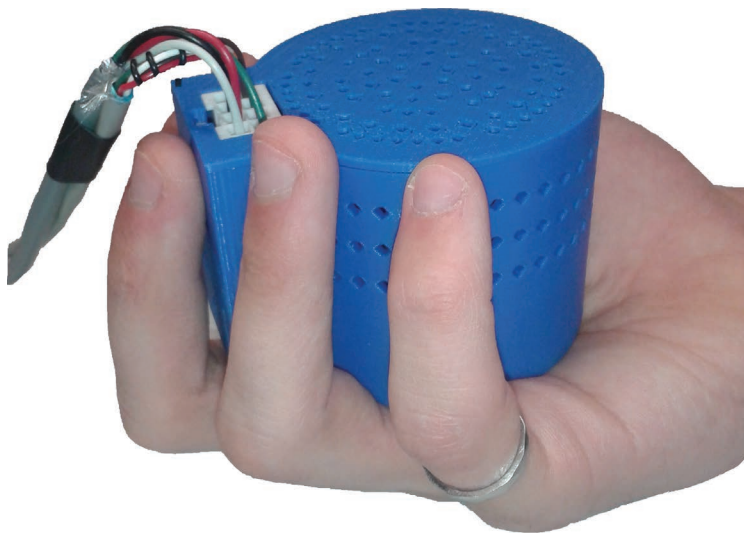
Figure 1. Handheld haptic compass for use as a navigation aid.
