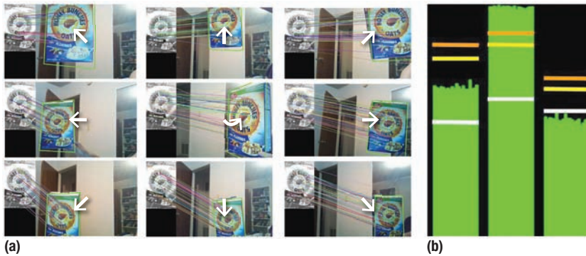
FIGURE 2. Version A of the Speeded up Robust Features (SURF) algorithm. (a) Directional commands (denoted by white arrows) through an audio channel guide the user so that the camera in the glasses can obtain at least a partial view of the product for matching. (b) Graph showing confidence levels for three product templates. Third Eye matches these points against points in the image template and assigns each match a confidence level, which it uses to decide if this is the desired product or if the user should move to another item. The horizontal colored lines represent threshold confidence levels.
