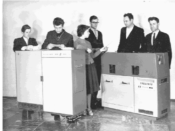
Fig. 4. The Rūta EVP 80-2. An original second-generation computer developed at the Special Computer Design Bureau in Vilnius and produced by the Vilnius Computer Factory. (From left to right) Members of the design team: Bronislovas Bieliauskas, Gediminas Zdanys, Jonas Puodžiū, Regina Valatkaite, Stanislovas Girlevičius, and Alfonsas Lipnickas.
