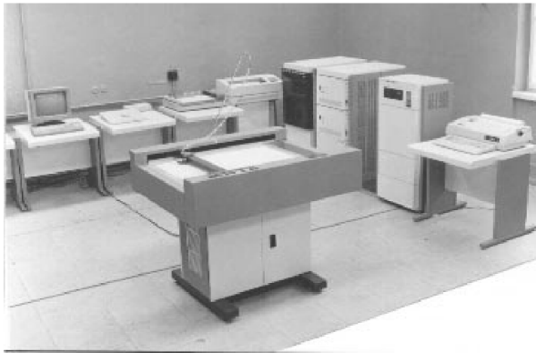
Fig. 6. The computer SM 1700, a VAX 730 clone, developed at the Special Computer Design Bureau in Vilnius and produced by Vilnius Computer Factory in 1986–1990.
