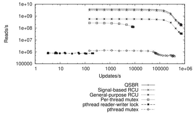
Fig. 13. Update Overhead, 64-core POWER5+, Logarithmic Scale
