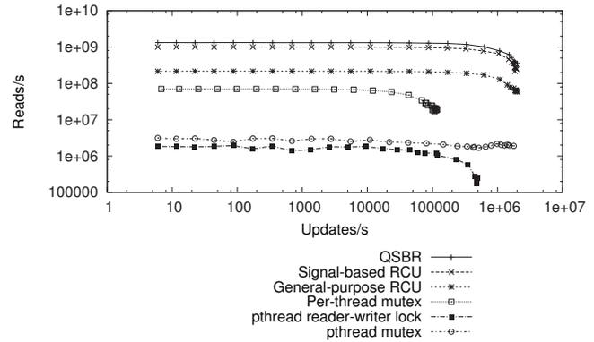
Fig. 12. Update Overhead, 8-core Intel Xeon, Logarithmic Scale
