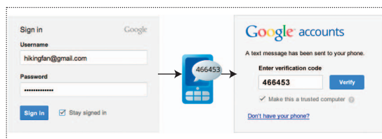
Figure 1. After successfully typing the right password during sign-in, the user enters a code from a preregistered mobile phone. The user can choose to skip the code next time on this particular browser.
