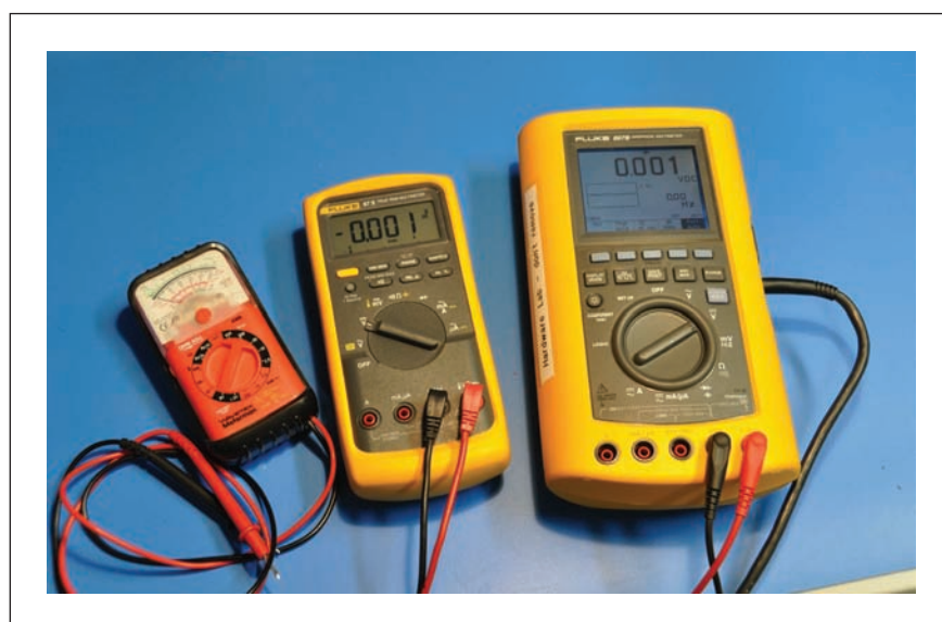
Figure 2. Evolution of a multimeter: an analog multimeter (left), a multimeter with LCD display (middle), and a multimeter with large screen display and analysis functions (right).
