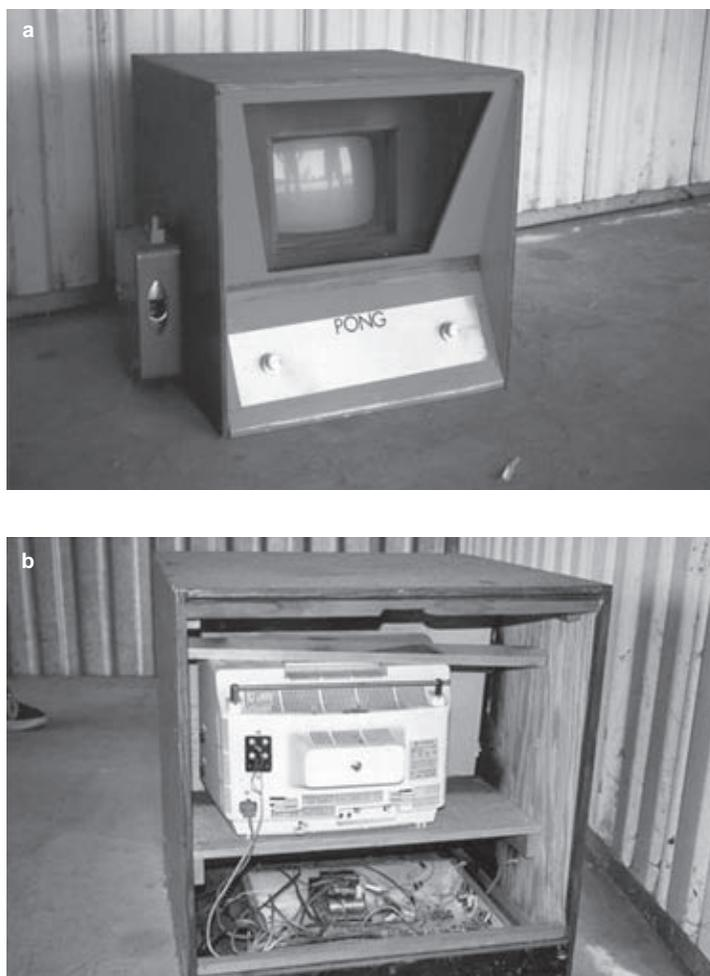
Figure 5. Pong prototype. (Photographs courtesy of Al Alcorn.)
