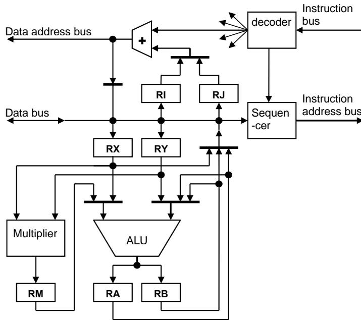
Figure 6. An efficient signal processor design of 1981 based on a freewheeling multiplier and dual accumulator achieved 10 million multiply-add per second.
