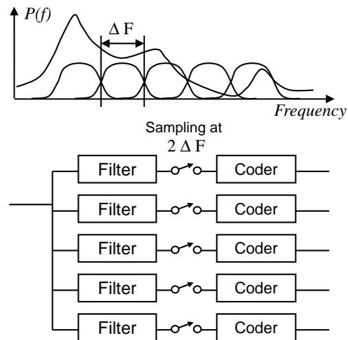
Figure 7. Coding audio signals in subbands.
