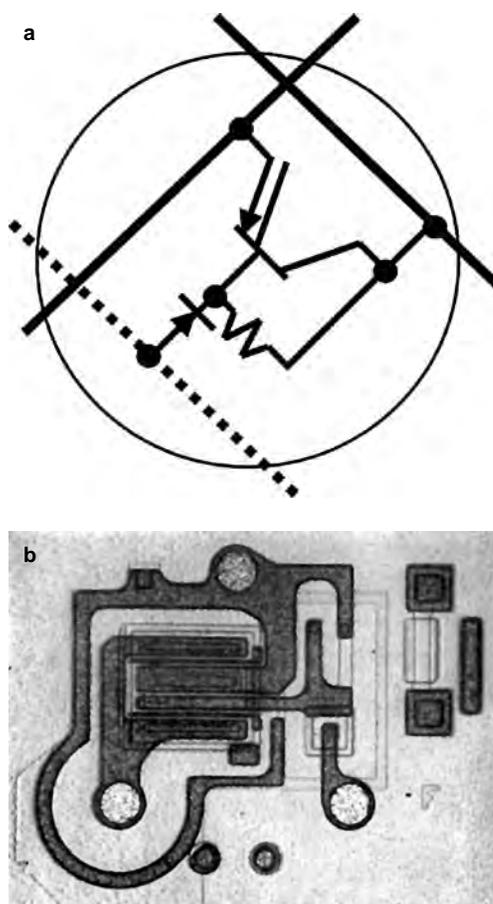
Figure 1. IBM 2750 PABX. (a) Circuit diagram and (b) microphotograph of its integrated cross point (die size approximately  $1 \text{ mm}^2$ ).
