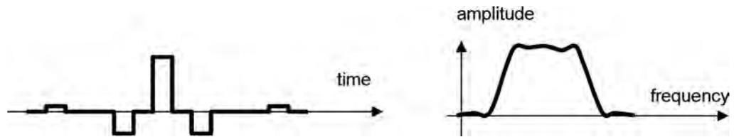
Figure 3. Pulse sequence and resulting spectrum from early digital echo modulator.
