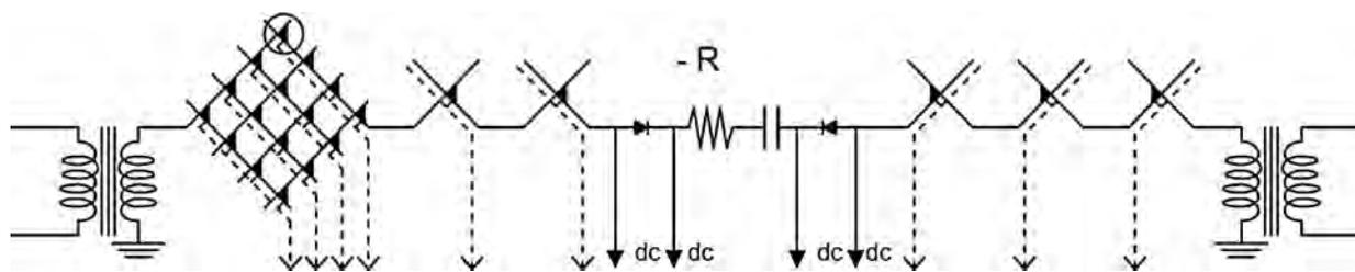
Figure 2. Simplified schematic diagram of the IBM 2750 unbalanced bidirectional switching network.
