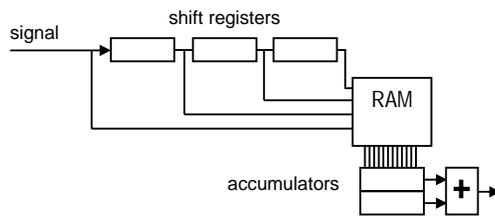
Figure 4. Digital multiplex filter (or distributed arithmetic)
