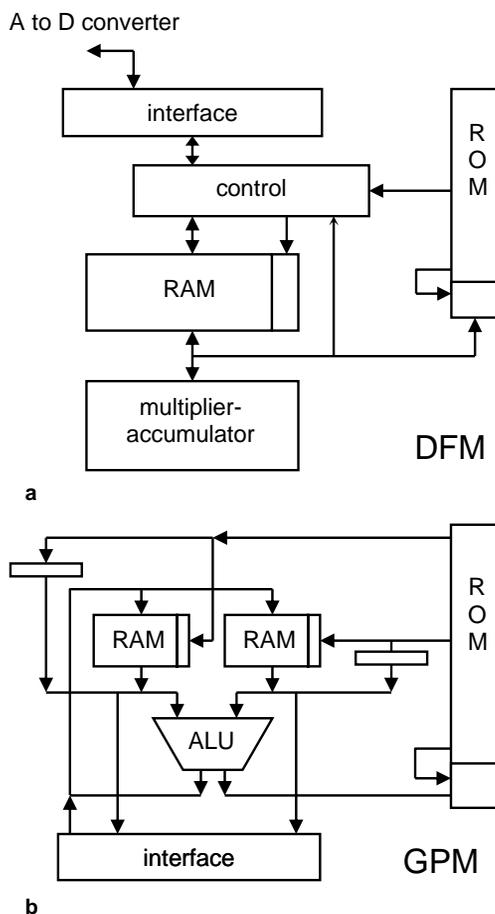
Figure 5. The first programmable signal processor introduced in 1976 comprised (a) separate arithmetic and (b) control elements.
